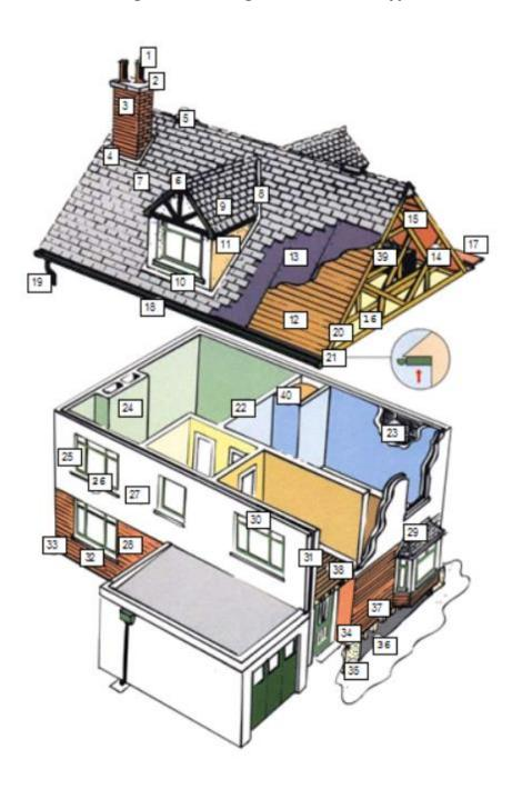
Chimney pots 2 Coping stone 3 Chimney head 4 Flashing Ridge ventilation 5 6 Ridge board Slates/tiles 8 Valley guttering 9 Dormer projection 10 Dormer flashing 11 Dormer cheeks 12 Sarking 13 Roof felt 14 Trusses 15 Collar 16 Insulation 17 Parapet gutter
